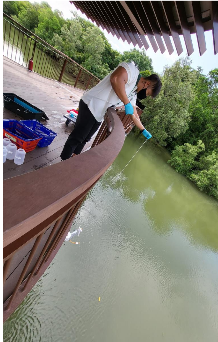
Horizontal water sampler used to collect seawater samples
