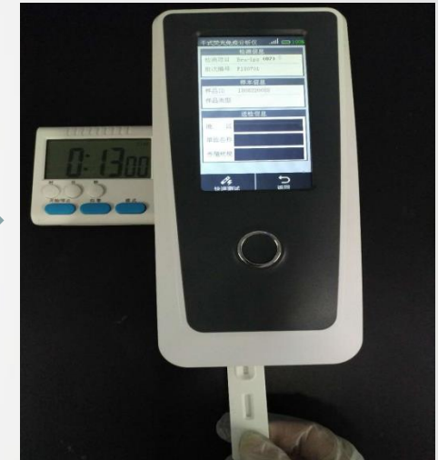
Reaction 15 minutes later on the computer to read the results, click the instrument to upload monitoring cloud platform network
