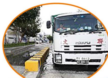
Disinfection pool for vehicles 進出車輛消毒池
